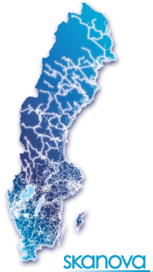
Fiber Network Covers 13 000 km of fiber optic cables, mostly buried along the railway - from Ålgården in the north to Helsingborg in the south with connections to Copenhagen and Oslo.
