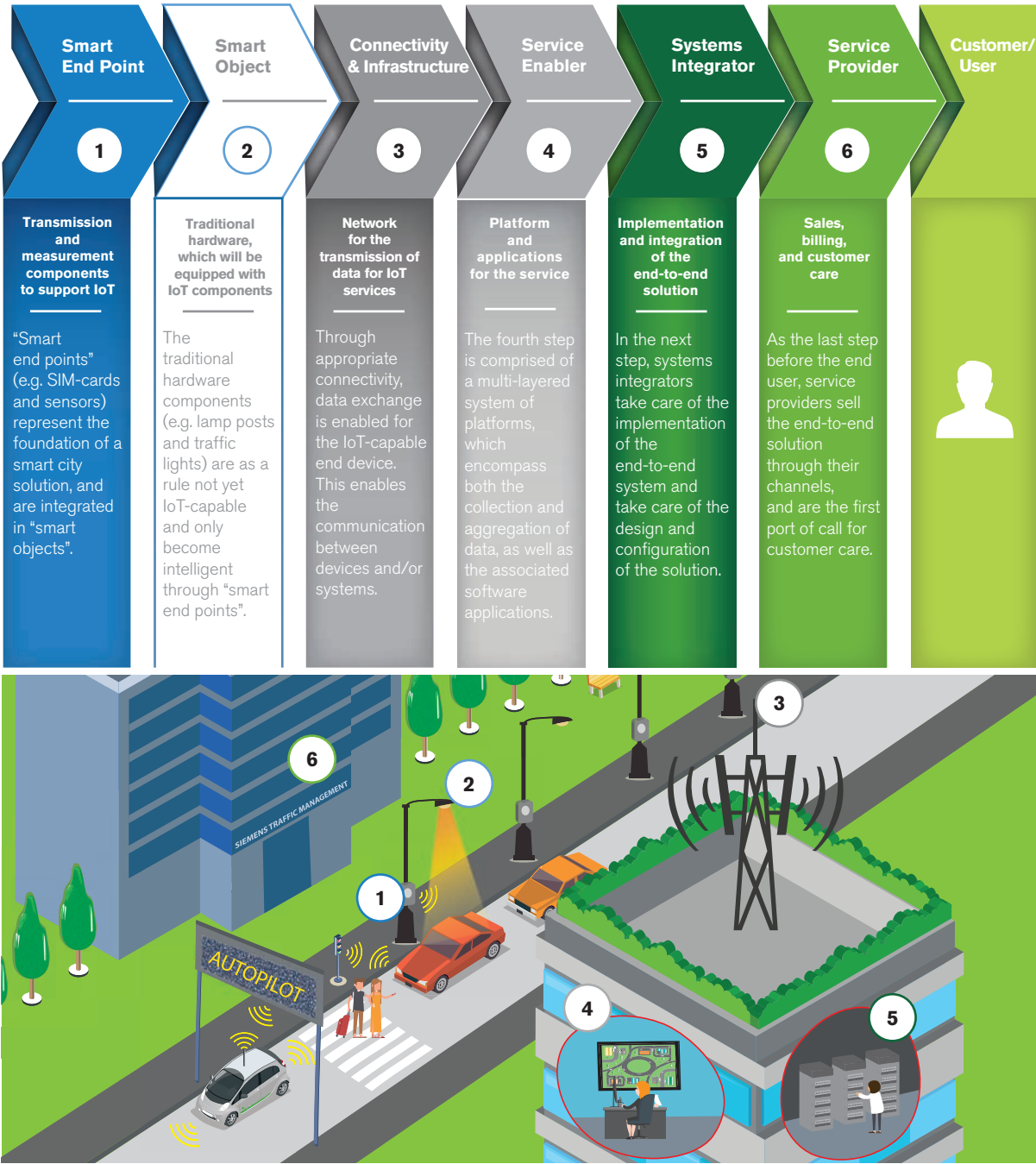
FIG. 6 The Smart City Value Chain – Using the Example of Data Exchange Between “Smart Street Lighting” and “Traffic Management”
